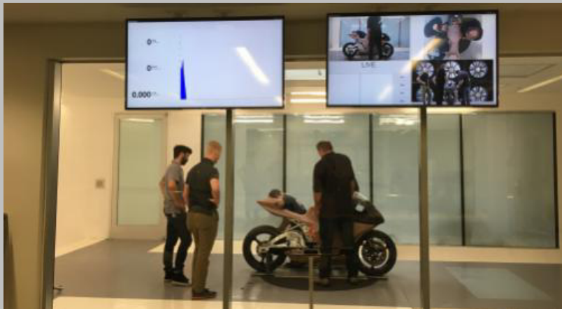
Lightning performs extensive aerodynamic wind tunnel and CFD (Computational Fluid Dynamics) testing.
